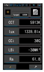
The TEXT screen displays user selected measurement values. Real time readings appear and are updated after every reading, next to their light measurement values.
