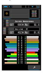
The CRI Comparison screen displays a percentage of the light source ability to reproduce a color accurately using the values (Ra, R1 to R15) with the comparison of two light sources next to each other.
