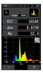
The Spectrum screen displays the spectral energy distribution of a source in real time. It can be displayed as a graph and data or full screen.
