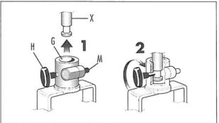
Unscrew knob "H", depress button "M", insert the male attachment "X" on the hole "G" and release the button. Lock firmly knob "H": ensure that the knob is able to seat in the recessed safety groove on the male attachment (fig. 10)
