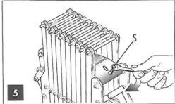
Insert the appropriate spring in housing "A" and block it with nuts "V" using appropriate wrench.
