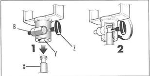
Unscrew knob "Z", depress button "B", insert the male attachment "X" on the hole "Y" and release the button. Lock firmly knob "Z": ensure that the knob is able to seat in the recessed safety groove on the male attachment (fig. 13)
