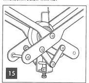
After mounting the load and firmly locked, secure it with appropriate safety cable (not supplied).
