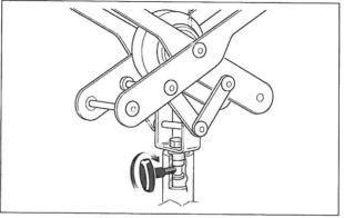
Always ensure that the knob of the 16mm (5(8") female attachment seat in the recessed safety groove on the pantograph 16mm (5/8") male attachment.
