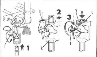
Loose knob "T" until 28 mm (1 1/8") luminair spigot can be fully inserted into the clamp. Insert the 28 mm (1 1/8") luminair spigot on the female attachment "R" until it protrudes as shown in figure 12.
